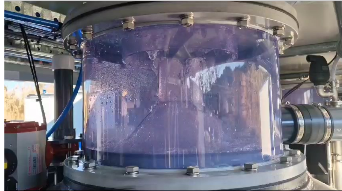
Primary Fractionation of raw groundwater
